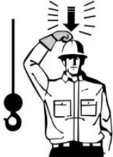
Figure I.5 UTILISER LE TREUIL PRINCIPAL
